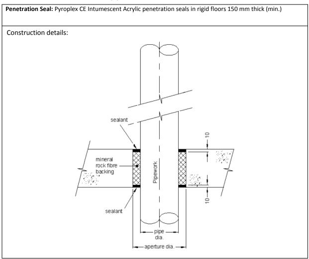
A.2.2.1 Pipes without insulation
