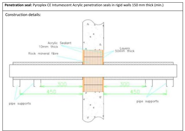
A.1.1.1 Pipes with local interrupted (minimum 500 mm) or continuous 19 mm thick Armacell 'Class O Armaflex' Insulation
