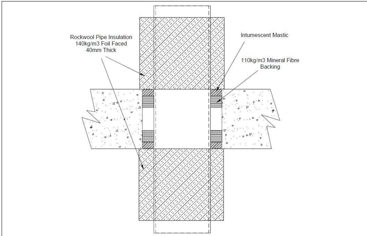
**A.3.3.1 Pipes with 40 mm thick/500 mm long, 140 kg/m<sup>3</sup> stone wool insulation**
